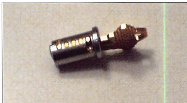
The original key, which uses shallower cuts in both the first and last position, allows the plug to rotate in both directions. This would be considered the "owner's key".
