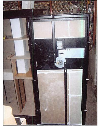
Photo 7 shows the door with an S&G 6741, this lock was pulled off a previous electronic upgrade.
