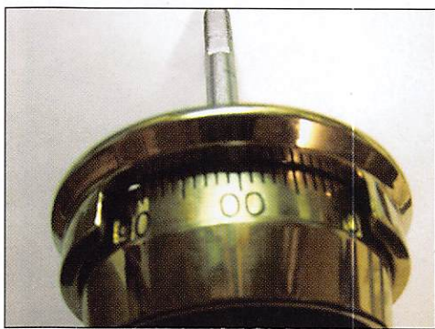
Photo 2 shows the original Amsec dial. Note that the dial starts at 00. All the current S&G dials start at 0, this is a quick way to tell which lock is installed.
